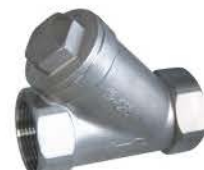
Y-type Female Strainer (CF8, CF8M, WCB) 1/4"~4" / 800PSI YS11F6N/800
