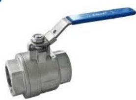
2PC Type Ball Valve Threaded Fire Safe (CF8, CF8M, WCB, Ti, Ni, LCC, LF2) 1/4"~4" / 2000PSI FBV12R6N/2000
